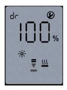
To change the open end-stop position, press the up/down arrows for the required position and press enter.
