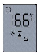
The top left function digits displays **CO** to indicate the supply air (changeover) temperature is being displayed. If no supply air sensor is connected the display will indicate zero.
