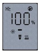
To manually drive the heater output, press the up/down arrows for the required percentage output and press enter.
