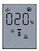
To manually drive the disk, press the up/down arrows for the required position and press enter.
