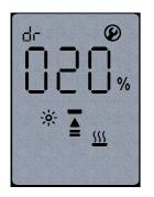
To change the close end-stop position, press the up/down arrows for the required position and press enter.
