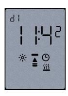
The watch icon will switch on to indicate the RTC function is selected. The current time, hh:mm will show. The top left function displays **dx**, with **x** being any digit between 1 and 7 to indicate the current day of the week. Monday is displayed as day 1. To edit the RTC, press the enter button and the minute display will flash. Select the current minute value with the up or down buttons. Press enter again and select the current hour. Enter again and select the current day.
