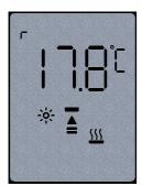
The top left function displays  $\mathbf{r}$  to indicate the remote (wall-stat) temperature is being displayed. This temperature is displayed regardless of temperature selection for control purposes.
